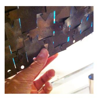
Figure 2. Proportions of details should be designed to accommodate the fabrication tool AND the assembly system.
