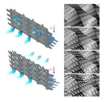
Figure 4. The diagram on the left demonstrates the self-ventilating capability of the Armoured Corset and the right shows the changing bimetal form on Bloom.
