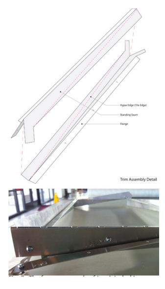
Figure 3. The frame was made of two interlocking, folded aluminum pieces.
