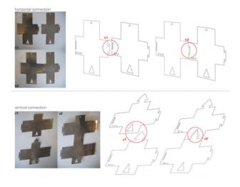
Figure 6. The tab-slot connection allowed for quick assembly and stabilization of the geometry.
